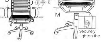
During assembly, hand tighten screws only. When the screws are in place, tighten completely.
