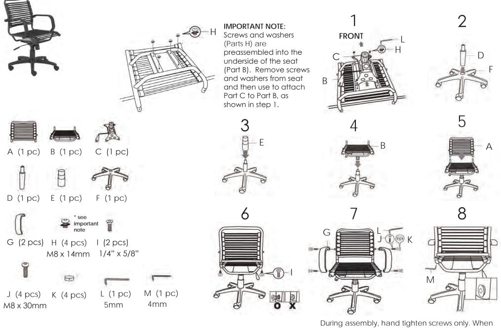
the screws are in place, tighten completely.
