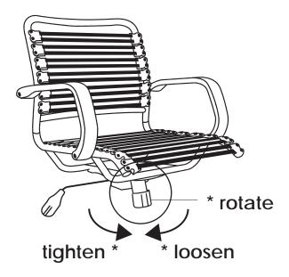
During assembly, hand tighten screws only. When the screws are in place, tighten completely.
