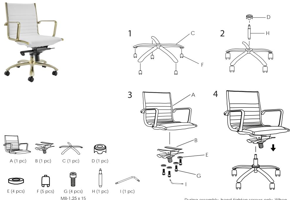
During assembly, hand tighten screws only. When the screws are in place, tighten completely.
