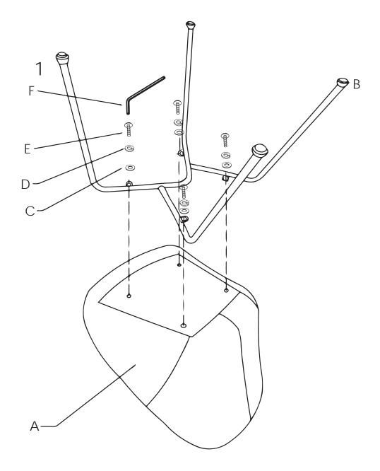
During assembly, hand tighten screws only. When the screws are in place, tighten completely.
