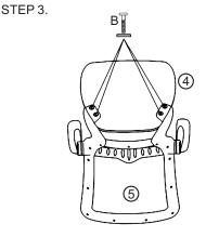
NOTICE: ATTACH BACK TO ARMS, AND FULLY TIGHTEN ALL SCREWS.
