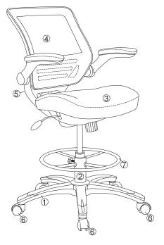
1 Base x1 2 Cylinder Column x1 3 Seat with Control Mechanism x1 4 Back Frame
