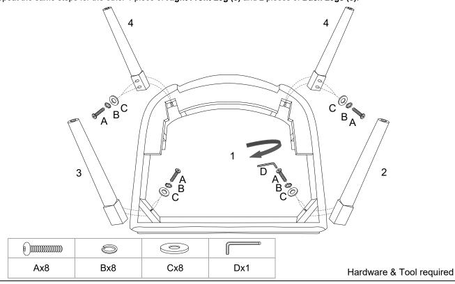
STEP 2: Carefully turn over the assembled **Chair Body (1)** as shown.
