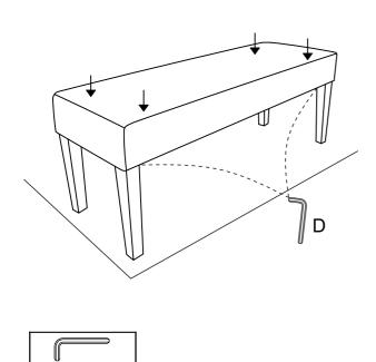
STEP3: Recover the Velcro on the bottom of **Seat Frame (1)**.
