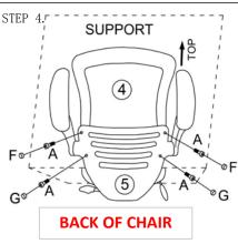
NOTICE: ATTACH BACK TO BACK SUPPORT, AND FULLY TIGHTEN ALL SCREWS.
