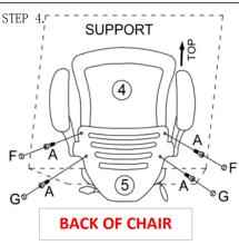
NOTICE: ATTACH BACK TO BACK SUPPORT, AND FULLY TIGHTEN ALL SCREWS.
