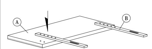
Align support board fixing holes over headboard fixing holes according to your desired height.
