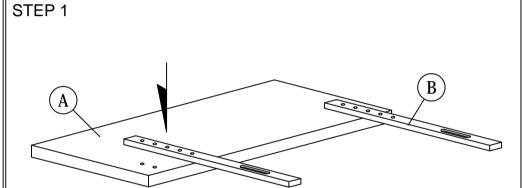
Align support board fixing holes over headboard fixing holes according to your desired height.
